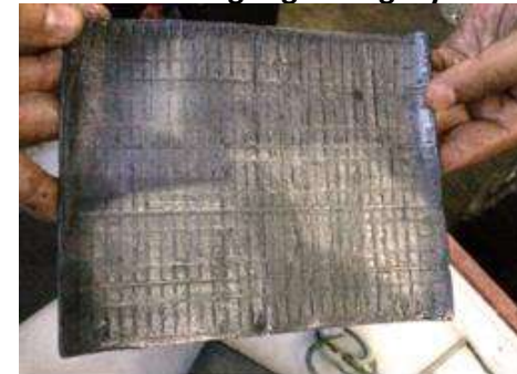
After Bend Test – MR Plate Showing High Integrity
